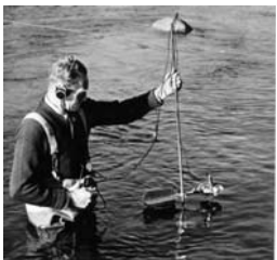
Traditional manner of taking current meter readings. In deeper water a boat is used.
