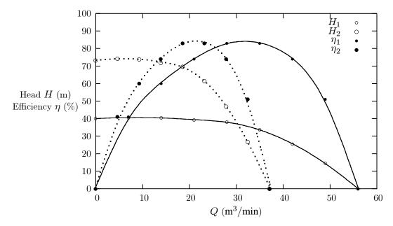
2. Consider a pump of characteristic diameter D = 0.4 m and rotational speed 1500 revolutions/min having the following data:
