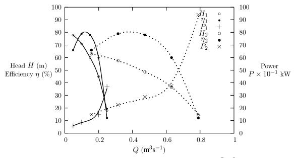
(d) From the graph of power required for the second pump, for  $0.55 \,\mathrm{m^3 \, s^{-1}}$ , about  $300 \,\mathrm{kW}$  would be required.
