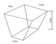
A mixing tank with trapezoidal ends is  $1.8 \text{ m} \log 0.9 \text{ m}$  deep and 0.9 m wide at the top, tapering to 0.3 m wide at the base. If the tank is completely filled with water, calculate
