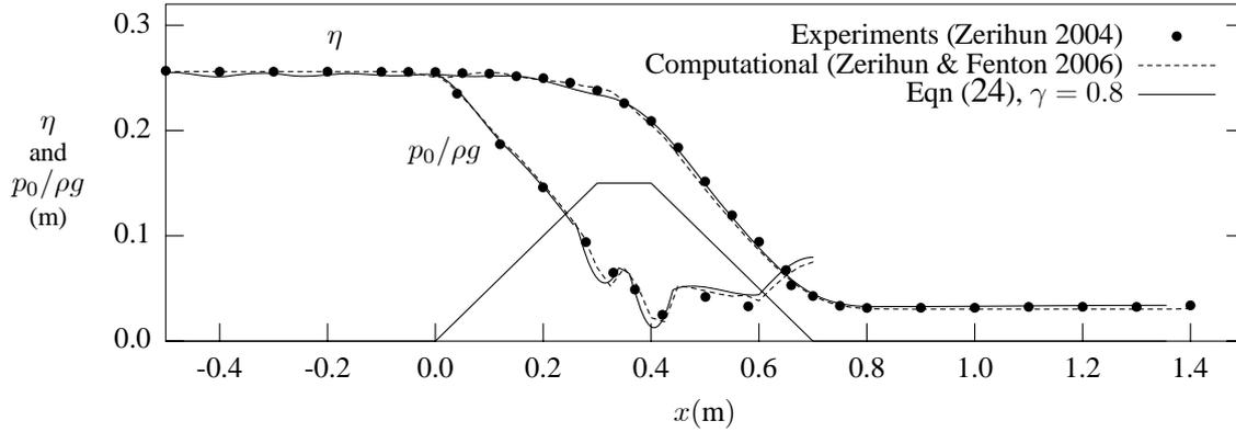
Figure 5. Flow over a short-crested trapezoidal weir
