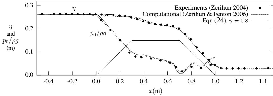
Figure 4. Flow over a broad-crested trapezoidal weir, showing surface elevation  $\eta$  and pressure head on the bed  $p_0/\rho g$
