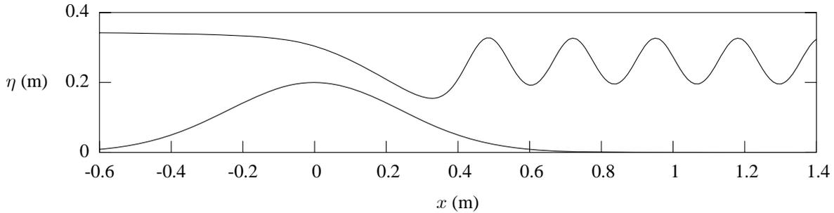
Figure 2. Computational results for the same flow as in Figure 1, but over a slightly lower hump, producing an undular hydraulic jump
