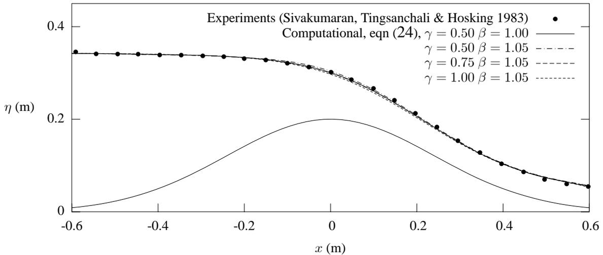
Figure 1. Steady flow over Gaussian hump, computational results for surface profile compared with experimental values of Sivakumaran et al. (1983)
