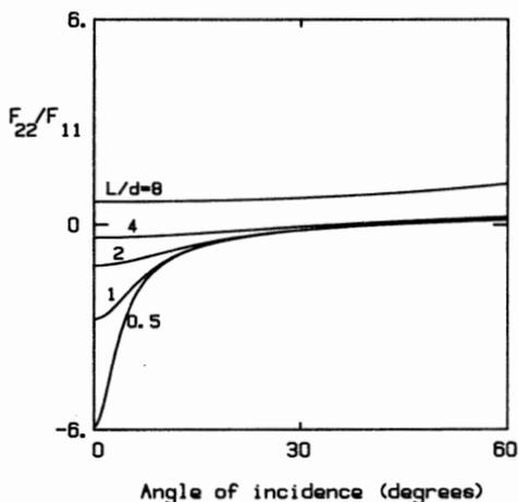
FIG. 1.—Relative Importance of Second-Order Coefficients, Expressed by Ratio  $F_{22}/F_{11}$ , and its Variation with Angle of Incidence and Relative Wavelength
