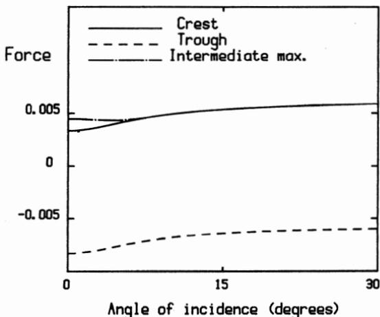
FIG. 2.—Variation of Force per Unit Length with Angle of Incidence for each of Three Parts of Wave, (1) for the Crest  $\chi = 0$ ; (2) for the Trough  $\chi = \pi$ ; and (3) for the Intermediate Maximum  $\chi_m$ . Values of the Force Plotted =  $P_*(\chi)/\rho g d^2$ ; the Whole Diagram is for the Case  $H_s/L = 0.05$ ;  $L/d = 1$
