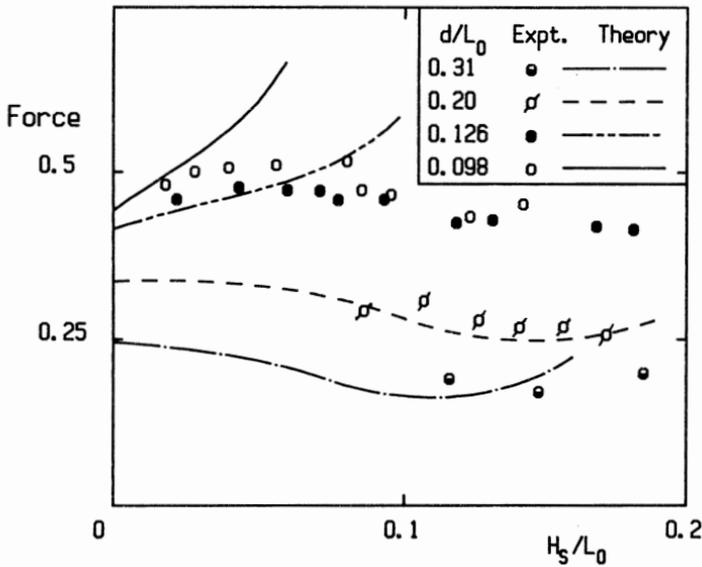
FIG. 5.—Comparison between Present Theory and Experimental Results of Goda; Value of Force Plotted is  $P_*/\rho g H_s d$
