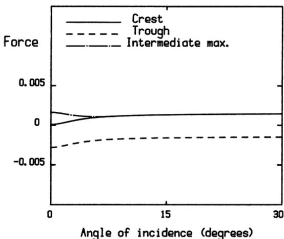
FIG. 3.—See Caption to Fig. 2; this Diagram is for the Same Relative Wave Height,  $H_s/L = 0.05$ , but for Shorter Waves,  $L/d = 0.5$
