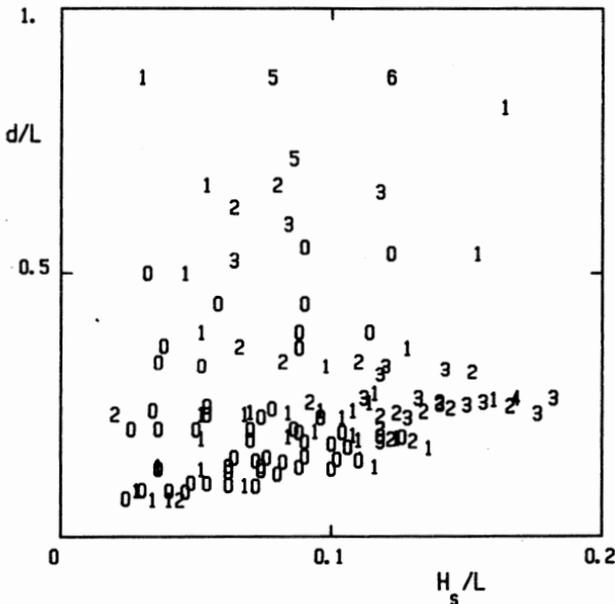
FIG. 4.—Comparison between Present Theory and Experimental Results of Nagai; each Number Shows Decile Difference between Theory and Experiment, thus "0" Means Less than 10% Difference, "1" Means 10–20%, etc.
