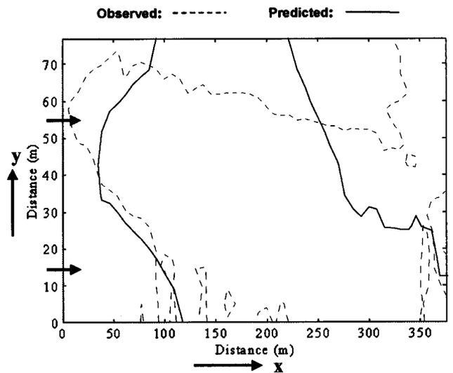
Fig. 15. Waterfront advance pattern in second basin after 30 min (arrows indicate direction of flow)
