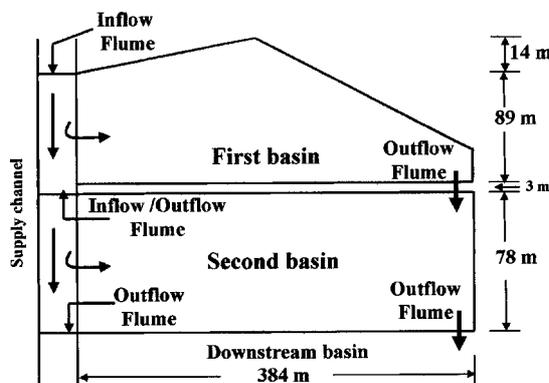
**Fig. 10.** Layout of multiple basins for validation
