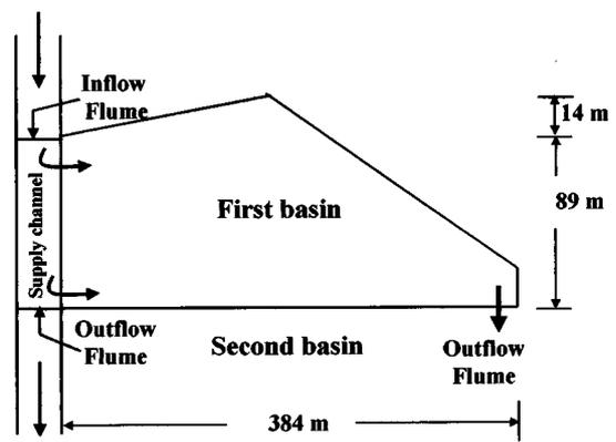
Fig. 6. Layout of single irregular shape contour basin
