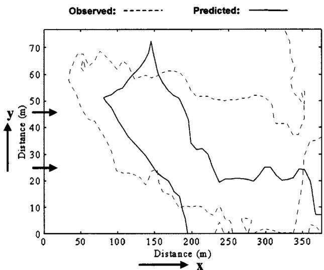
Fig. 16. Waterfront advance in second basin after 1 h (arrows indicate direction of flow)
